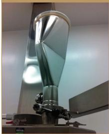
A double transition hopper design was adopted to improve the flow properties of the granulation. This design provided flow along the walls (mass flow) based on wall friction results and minimizing arching potential, based on cohesive strength results. This hopper design was "more robust," with respect to providing mass flow, than a simple conical hopper.
