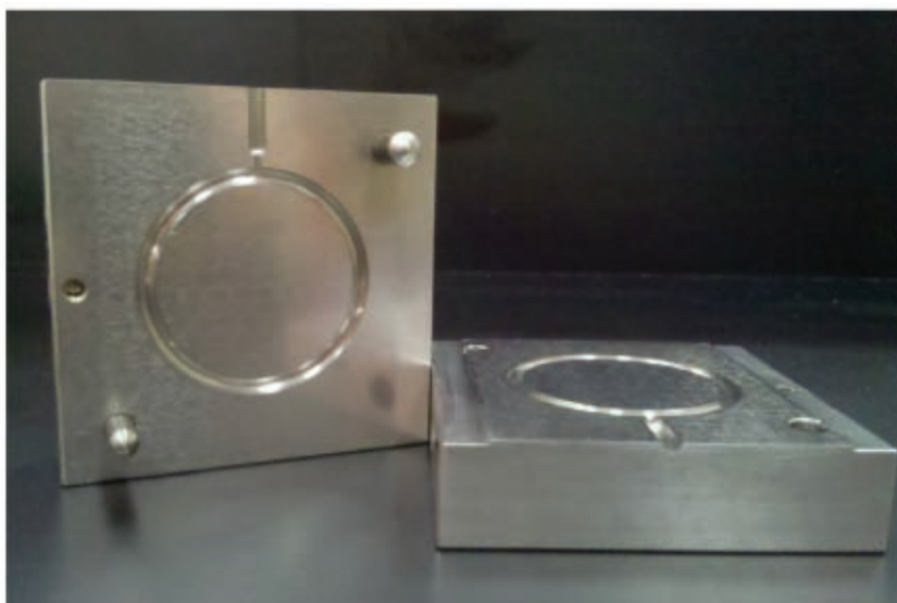
A simple aluminum o-ring mold showing both mold halves. The cold-runner that feeds the cavity is the channel at the top of the upper-right half.
