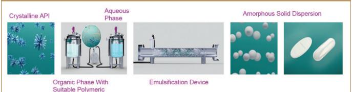
Microparticle Process for the Formation of Ready-to-Fill ASDs
