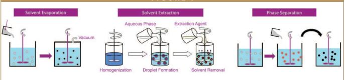
**Different Types of Microparticle Encapsulation Technologies**
