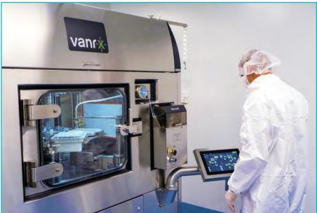
Eurofins scientist using Microcell Vial Filler for sterile fill/finit
